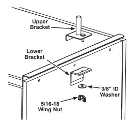
4. Assemble the rod assembly to the post of the upper bracket assembly as shown by adjusting the wing nut.
